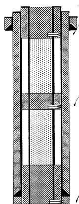
4. PUH & perf @ 355' & sqz 100 sx Class "C" cmt from 355' to surf, CIRC 8 5/8" to surf. (Surf Shoe & Water Board)
