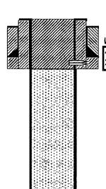
4. PUH & perf @ 250' & sqz 225 sx Class "C" cmt from 250' to surf, CIRC 7"to surf. (Water Board)
