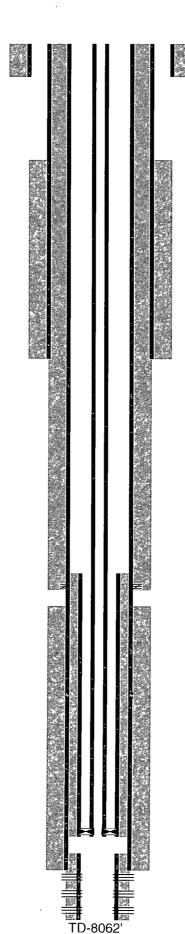
17-1/2" hole @ 306' 13-3/8" csg @ 306' w/ 350sx-TOC-Surf-Circ
