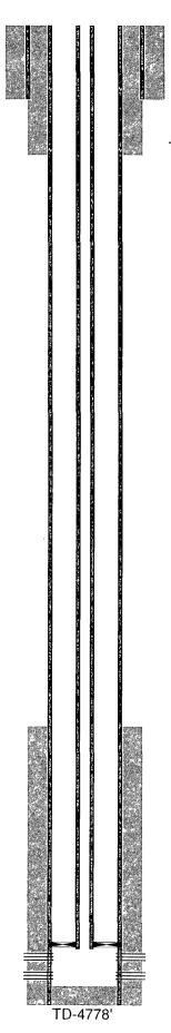
12-1/4" hole @ 367' 8-5/8" csg @ 367' w/ 263sx-TOC-Surf-Circ
