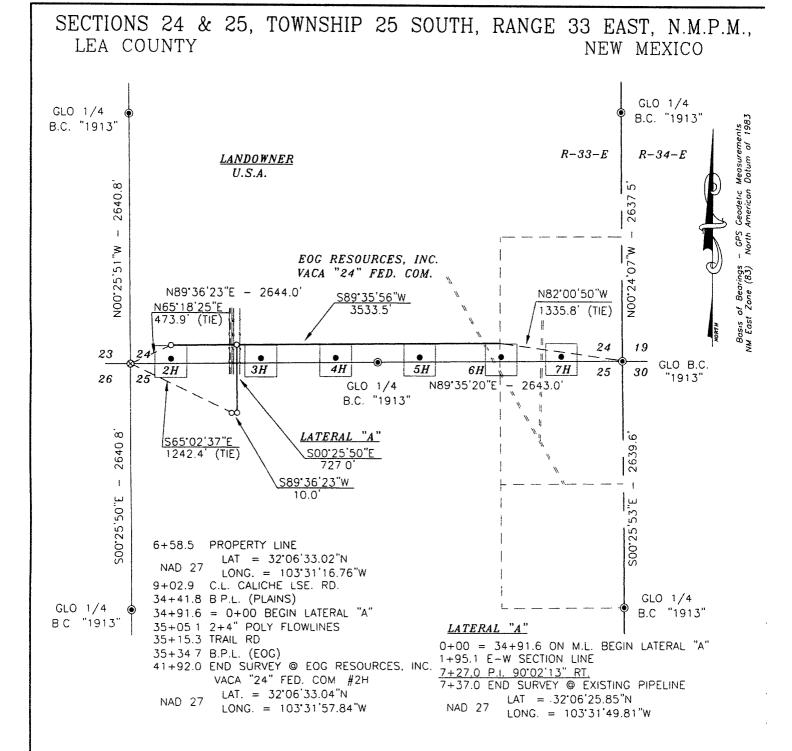
STRIP OF LAND 30.0 FEET WIDE AND 4270.5 FEET OR 0.809 MILES IN LENGTH CROSSING U.S.A. LAND IN SECTIONS 24 & 25, TOWNSHIP 25 SOUTH, RANGE 33 EAST, N M P.M., LEA COUNTY, NEW MEXICO AND BEING 15.0 FEET LEFT AND 15 0 FEET RIGHT OF THE ABOVE PLATTED CENTERLINE SURVEY.
