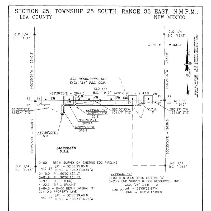
A STRIP OF LAND 30.0 FEET WIDE AND 3233.2 FEET OR 0.612 MILES IN LENGTH CROSSING U.S.A. LAND IN SECTION 25, TOWNSHIP 25 SOUTH, RANGE 33 EAST, N.M.P.M., LEA COUNTY, NEW MEXICO AND BEING 15.0 FEET LEFT AND 15.0 FEET RIGHT OF THE ABOVE PLATTED CENTERLINE SURVEY
