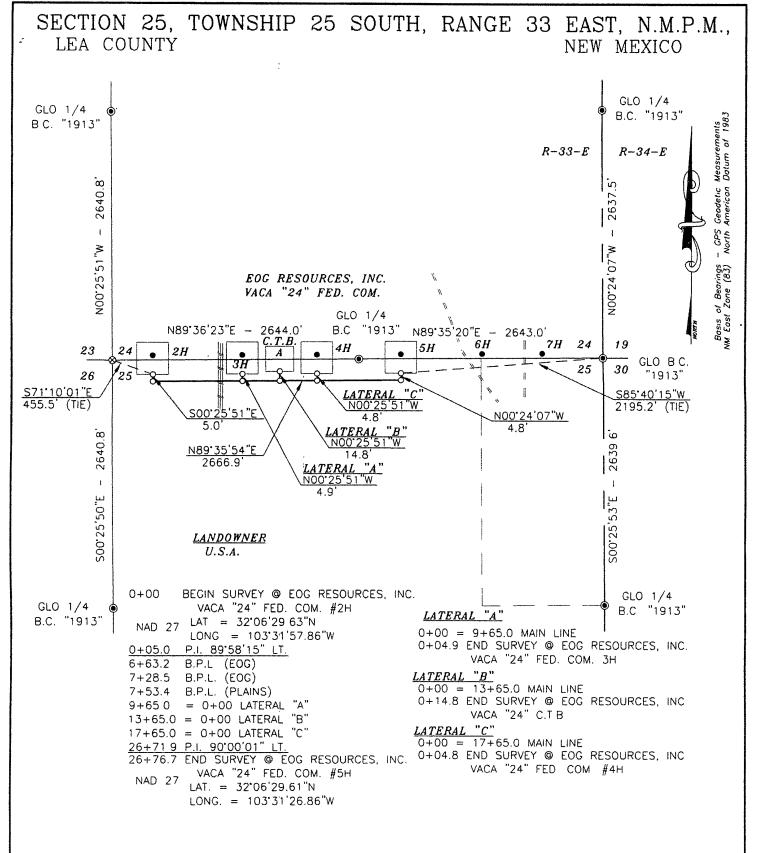
A STRIP OF LAND 30.0 FEET WIDE AND 2701 2 FEET OR 0.512 MILES IN LENGTH CROSSING U.S.A. LAND IN SECTION 25, TOWNSHIP 25 SOUTH. RANGE 33 EAST, N.M.P.M., LEA COUNTY, NEW MEXICO AND BEING 15.0 FEET LEFT AND 15.0 FEET RIGHT OF THE ABOVE PLATTED CENTERLINE SURVEY.
