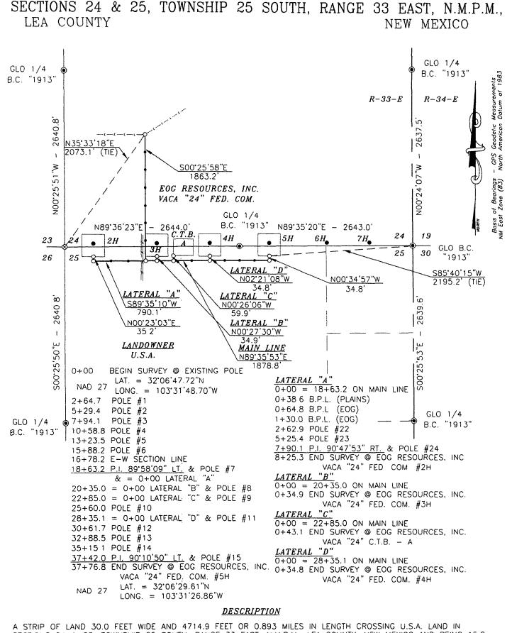
A STRIP OF LAND 30.0 FEET WIDE AND 4714.9 FEET OR 0.893 MILES IN LENGTH CROSSING U.S.A. LAND IN SECTIONS 24 & 25, TOWNSHIP 25 SOUTH, RANGE 33 EAST, N.M.P.M., LEA COUNTY, NEW MEXICO AND BEING 15.0 FEET LEFT AND 15.0 FEET RIGHT OF THE ABOVE PLATTED CENTERLINE SURVEY.
