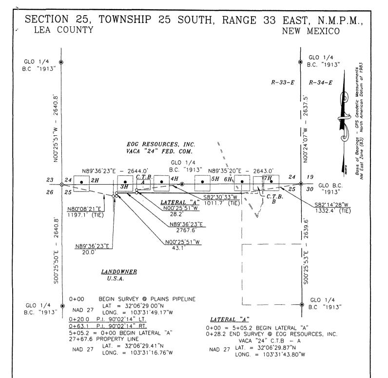
A STRIP OF LAND 30.0 FEET WIDE AND 2792.8 FEET OR 0.529 MILES IN LENGTH CROSSING U.S.A. LAND IN SECTION 25, TOWNSHIP 25 SOUTH, RANGE 33 EAST, N.M.P.M., LEA COUNTY, NEW MEXICO AND BEING 15.0 FEET LEFT AND 15.0 FEET RIGHT OF THE ABOVE PLATTED CENTERLINE SURVEY
