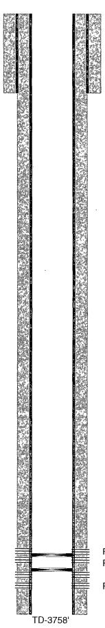
11" hole @ 510' 8-5/8" csg @ 510' w/350sx-TOC-Surf-Circ
