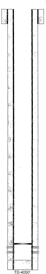
11" hole @ 265' 8-5/8" csg @ 265' w/ 125sx-TOC-Surf-Circ
