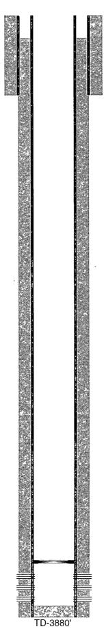
13-3/8" hole @ 410' 9-5/8" csg @ 410' w/ 250sx-TOC-Surf-Circ
