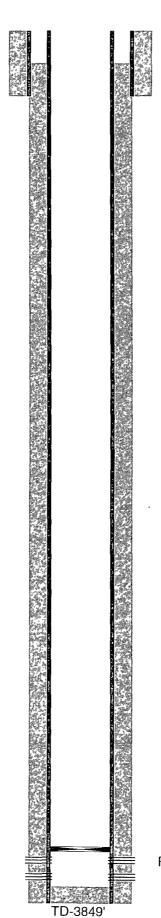
11" hole @ 318' 8-5/8" csg @ 318' w/ 300sx-TOC-Surf-Circ
