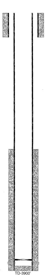
12-1/4" hole @ 370' 8-5/8" csg @ 370' w/ 300sx-TOC-Surf-Circ
