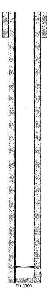
11" hole @ 369' 7-5/8" csg @ 369' w/ 200sx-TOC-Surf-Circ
