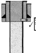
3. PUH & perf @ 364' & sqz 130 sx Class "C" cmt from 364' to surf, CIRC 7" to surf (Shoe & Water Board)
