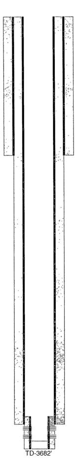
9-7/8" hole @ 1205' 7-5/8" csg @ 1205' w/ 500sx-TOC-Surf-Circ
