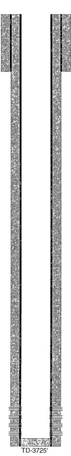
11" hole @ 500' 8-5/8" csg @ 500' w/ 300sx-TOC-Surf-Circ
