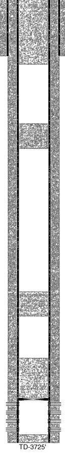
7-7/8" hole @ 3725' 5-1/2" csg @ 3725' w/ 1100sx-TOC-Surf-Circ
