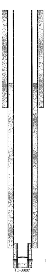
12-1/4" hole @ 1430' 8-5/8" csg @ 1430' w/ 730sx-TOC-Surf-Circ
