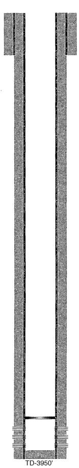
11" hole @ 399' 8-5/8" csg @ 399' w/ 300sx-TOC-Surf-Circ
