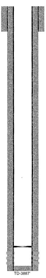
12-1/4" hole @ 372' 8-5/8" csg @ 372' w/ 350sx-TOC-Surf-Circ
