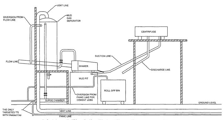
The flare discharge must be 100' from wellhead for non H2S wells and 150' from wellhead for wells expected to encounter H2S.
