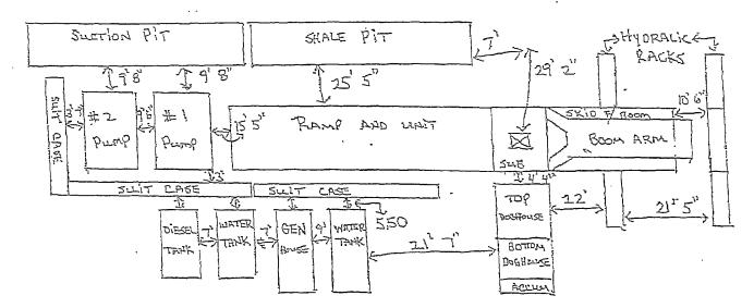
CENTER OF HOLE TO BACK OF STEEL PITS 40 CENTER OF HOLE TO END OF ACCUMULATOR 61, CENTER OF HOLE TO END OF WHIT RAMP 58 CENTER OF HOLE TO END OF BOOM - 44, CENTER OF HOLE TO END OF BOOM - 44, CENTER OF HOLE TO END OF SKID FOR BOOM - 34,
