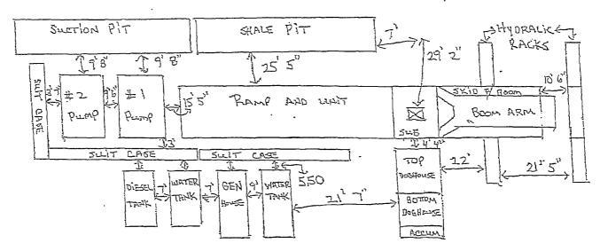
CENTER OF HOLE TO BACK OF STEEL PITS 40 CENTER OF HOLE TO END OF ACCUMULATOR 61, CENTER OF HOLE TO END OF WHIT RAMP 58 CENTER OF HOLE TO END OF BOOM - 44, CENTER OF HOLE TO END OF BOOM - 34, CENTER OF HOLE TO END OF SKID FOR ROOM - 34,
