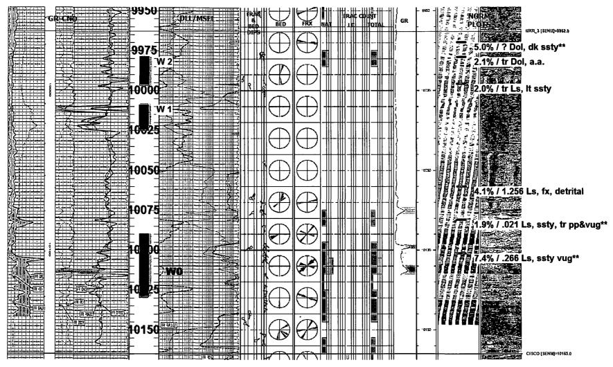
Similarly, these lower Wolfcamp zones should be perforated across the three intervals with the blue bars. The lowest recommended perforation interval (W0) has been added on the basis of the density of fracturing, and primary porosities in core up to 7.4%. The fractures would serve to effectively inter-connect porosity across the interval.
