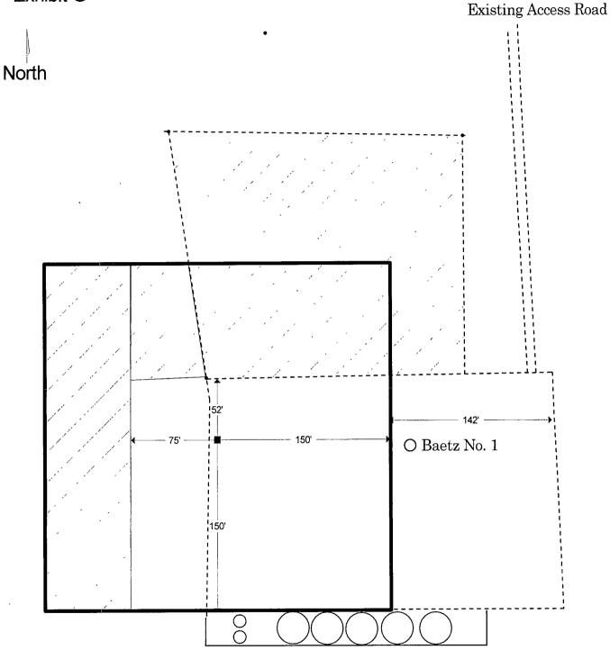
Old reserve pit will be dug up and remediated. Hatched areas are areas of interim reclamation. There will be 4 oil tanks, 1 water tank, a seperator, and a heater treater.
