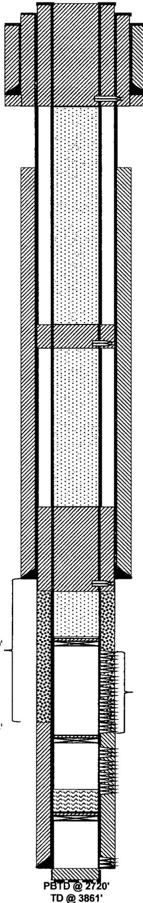
3. PUH & perf @ 286' & sqz 200 sx Class "C" cmt from 286' to surf, CIRC all strings to surf. (Shoe & Water Board)
