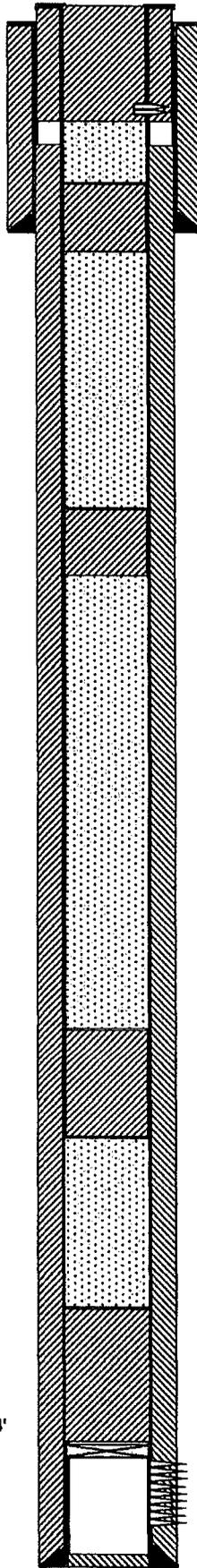
6. PUH & perf @ 150' & sqz 50 sx Class "C" cmt from 150' to surf, CIRC 5 1/2" to surf. (Water Board)
