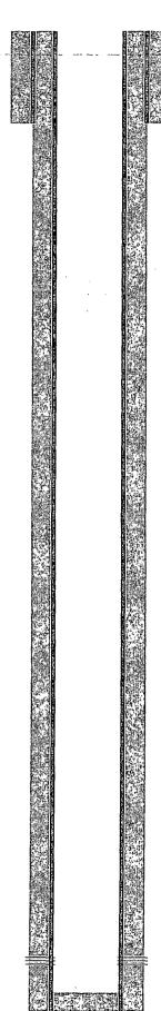
12-1/4" hole @ 394' 8-5/8" csg-@-394' w/ 300sx-TOC-Surf-Circ
