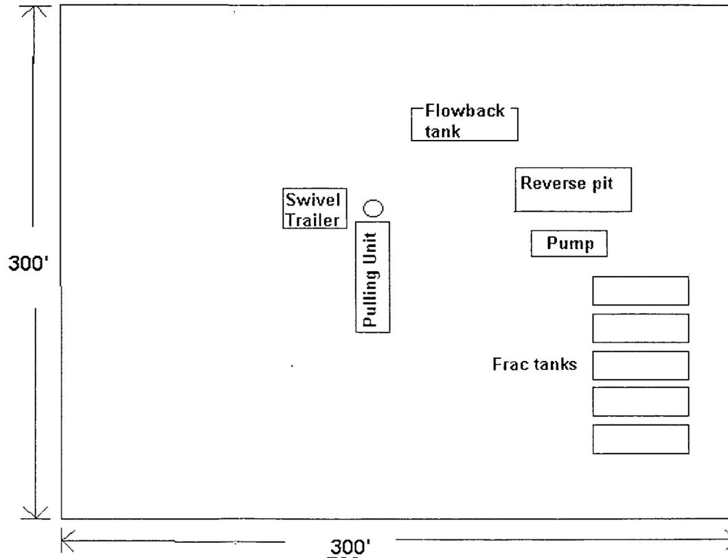
Note: Flowback tank is a frac tank, Reverse pit is a steel open top tank measuring 20' L x 7' W x 6' D.
