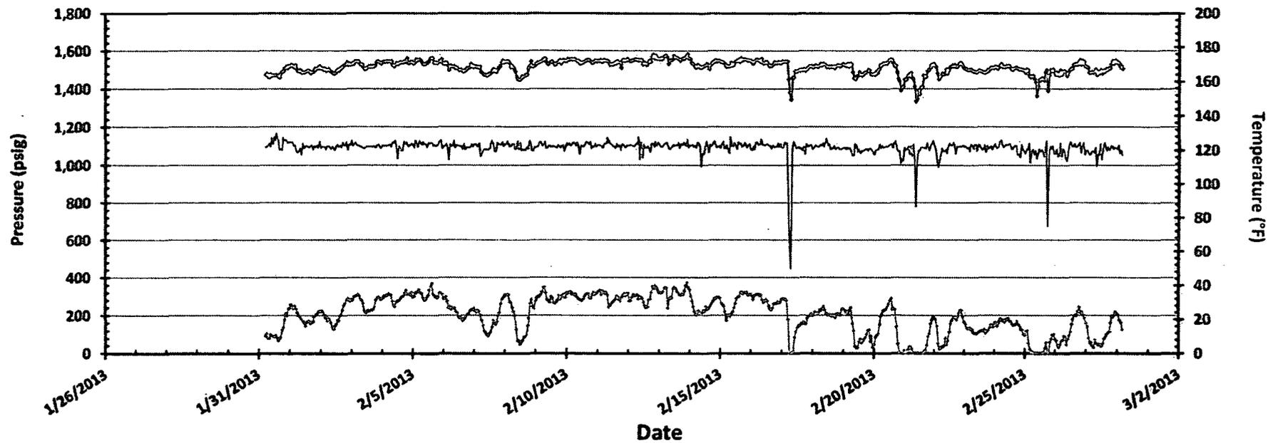
Linam AGI #1 TAG Injection Pressure and Casing Annular Pressure Differential (psig) 1/31/2013 to 2/28/2013
