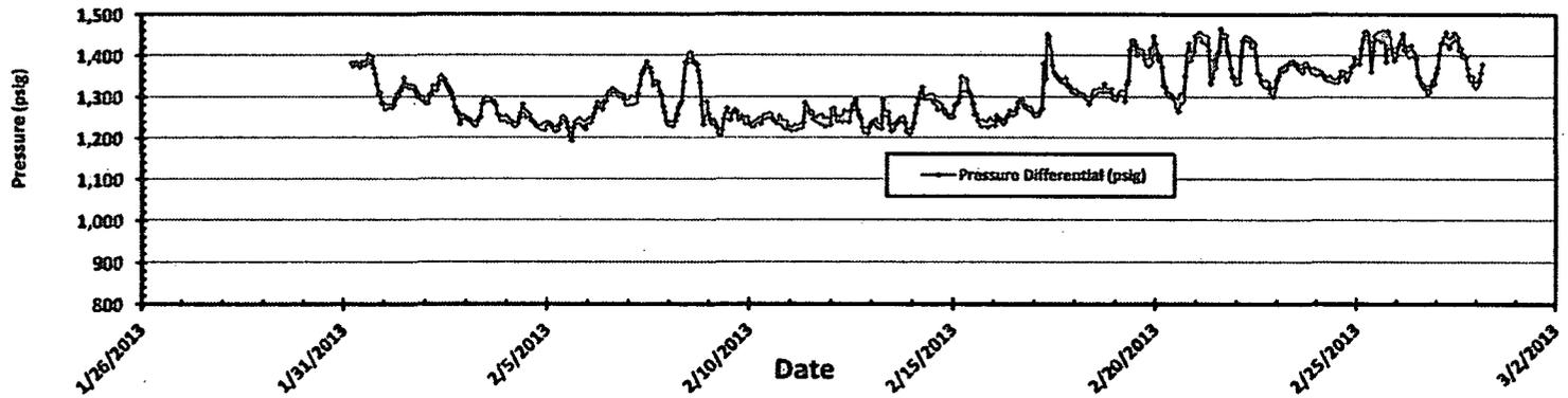
Linam AGI #1 TAG Injection Pressure and Casing Annular Pressure Differential (psig) 1/31/2013 to 2/28/2013
