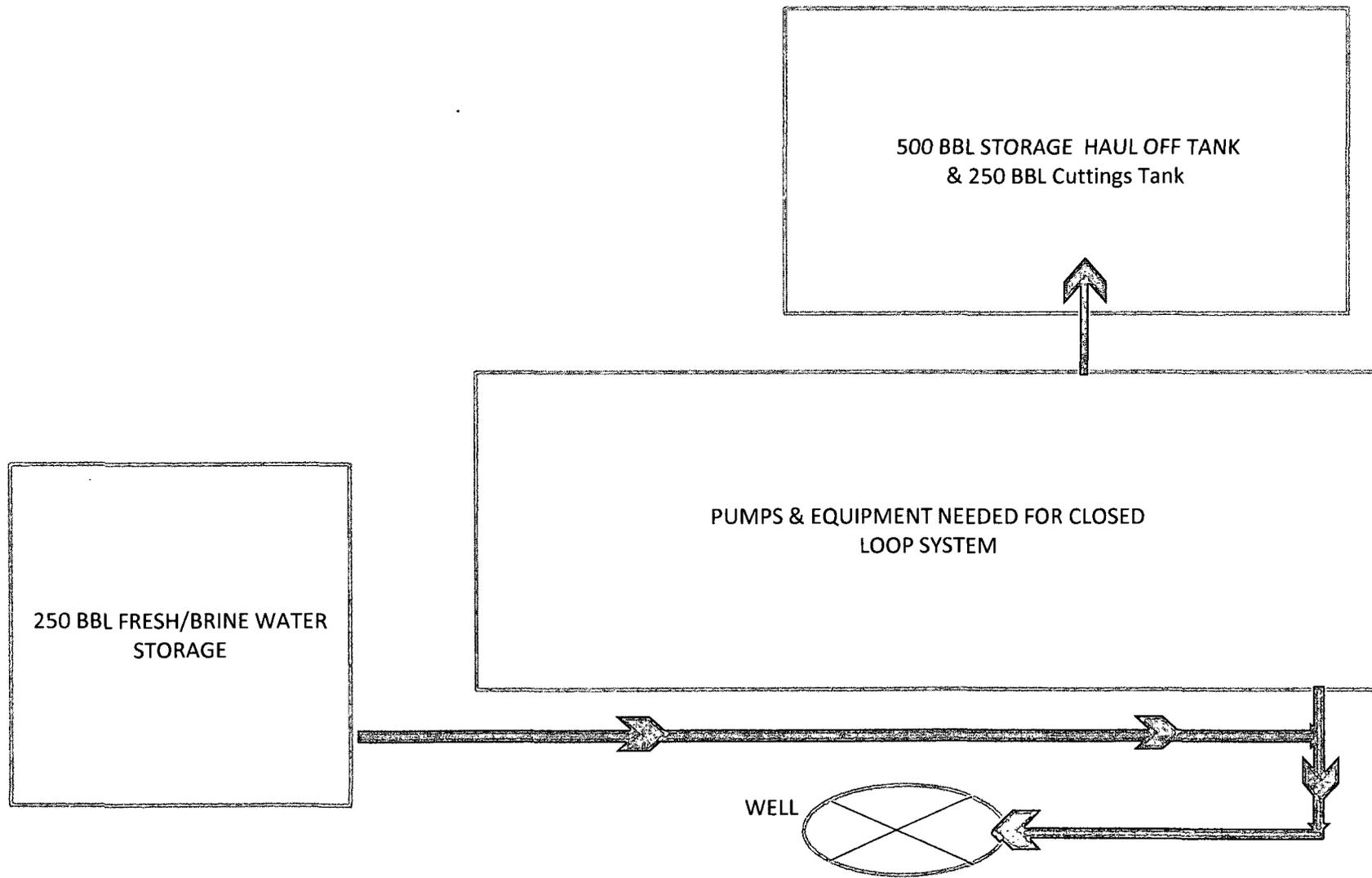
CLOSED LOOP DESIGN PLAN FOR PLUG BACK, SWD CONVERSION, DEEPENING, RE-COMPLETIONS, P&A, T&A OPERATIONS
