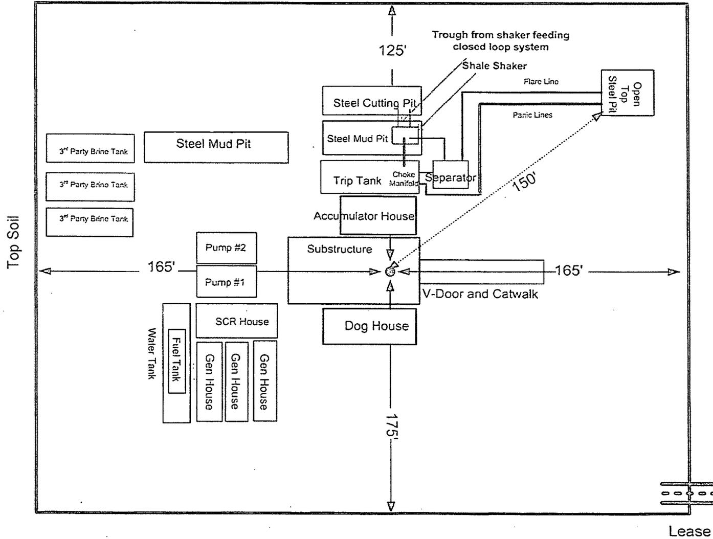
The Flare Line(s) Discharge Shall Be Located Not Less Than 100 Feet From The Wellhead, Having Straight Lines Unless Turns Are Targeted With Running Tees, And Shall Be Positioned Downwind From The Prevailing Wind Direction And Shall Be Anchored.
