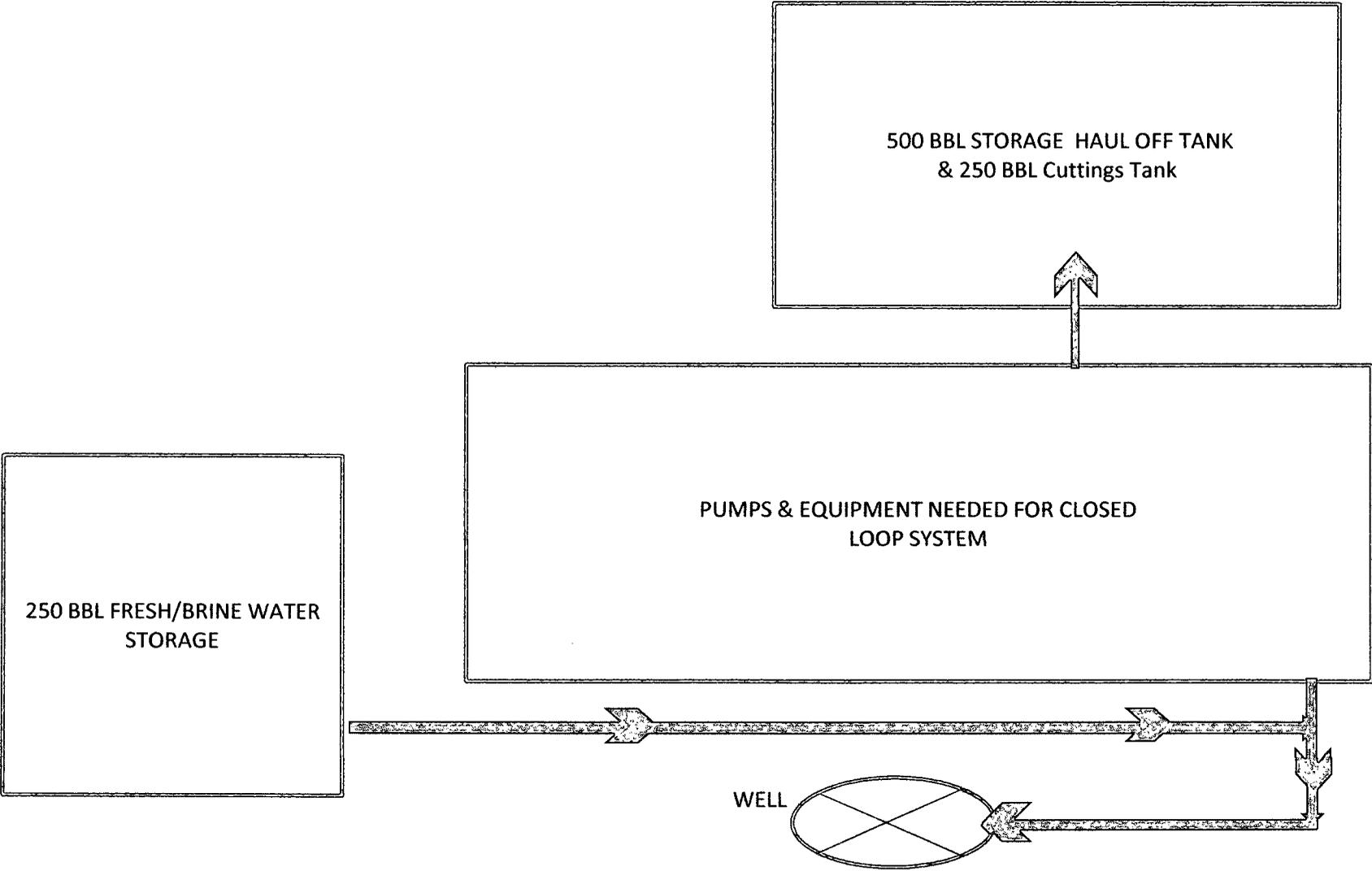
CLOSED LOOP DESIGN PLAN FOR PLUG BACK, SWD CONVERSION, DEEPENING, RE-COMPLETIONS, P&A,
