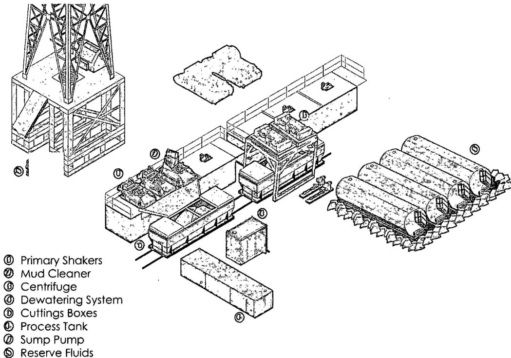
**Centrifuges:** The centrifuges can be utilized depending on the well's anticipated solids volume. One or two centrifuges can be used depending on the well geometry or depth of well. The centrifuges are sized to maintain low gravity solids at 5% or below. They may or may not need a dewatering system to enhance the removal rates. The centrifuges can make a cut point of 8-10 microns depending on bowl speed, feed rate, solids loading and other factors.
