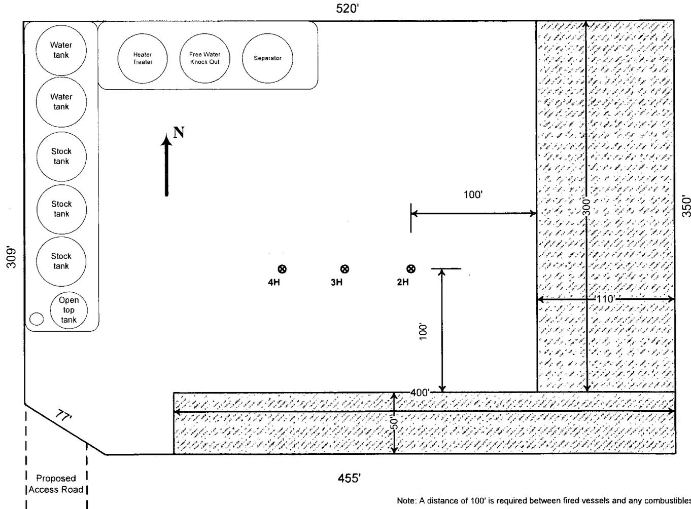
Note: A distance of 100' is required between fired vessels and any combustibles for safety purposes.
