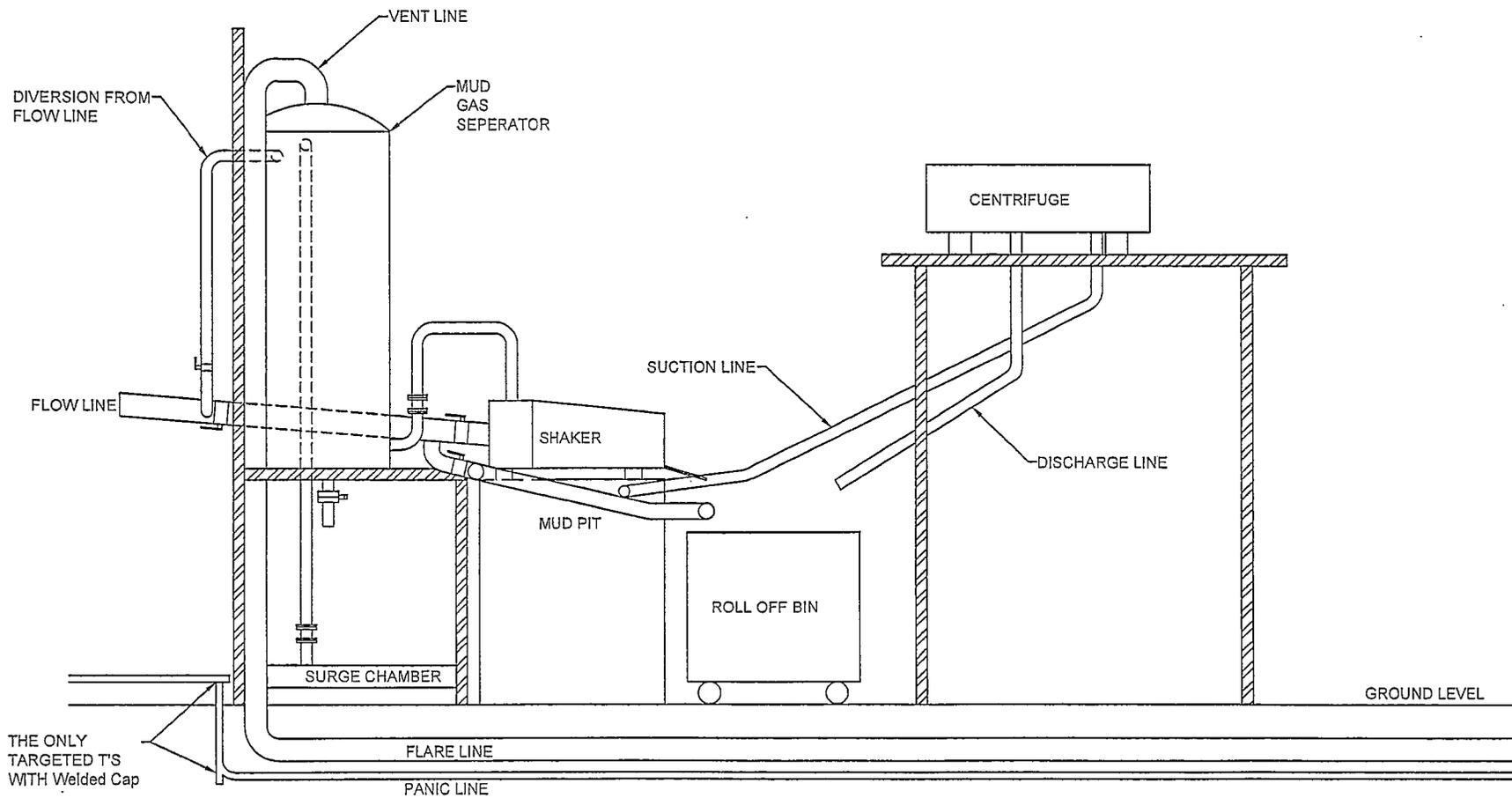
The flare discharge must be 100' from wellhead for non H<sub>2</sub>S wells and 150' from wellhead for wells expected to encounter H<sub>2</sub>S.
