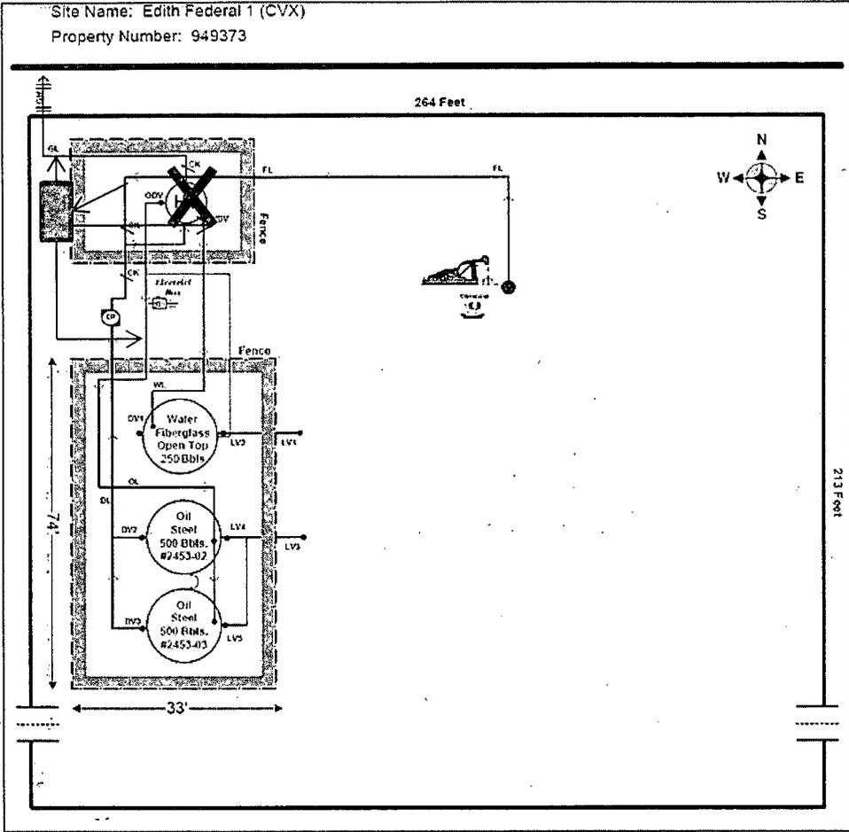
Due to High line pressure , we will add temporary 3 phase separator (denoted by blue square) to bypass the HT (denoted by the big X as bypassed). Once the line pressure is back to normal, we will remove the temporary separator and use existing facility. Like before. Expected duration of temporary solution is 6 months
