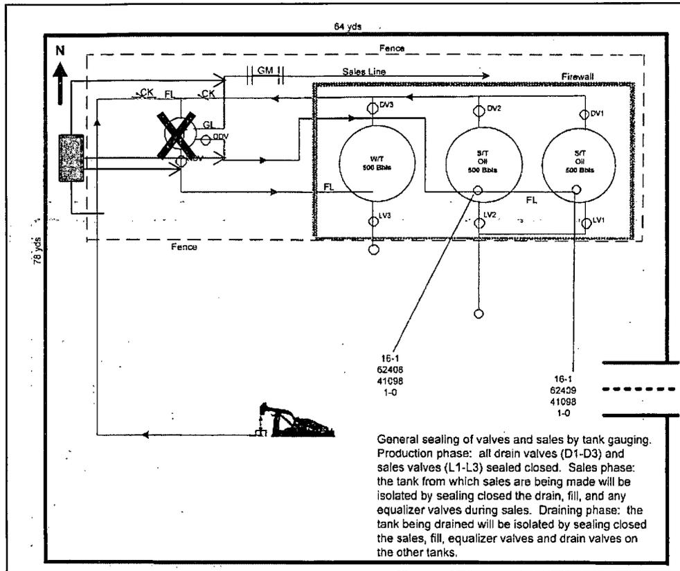
Due to High line pressure , we will add temporary 3 phase separator (denoted by blue square) to bypass the HT (denoted by the big X as bypassed). Once the line pressure is back to normal, we will remove the temporary separator and use existing facility. Like before. Expected duration of temporary solution is 6 months
