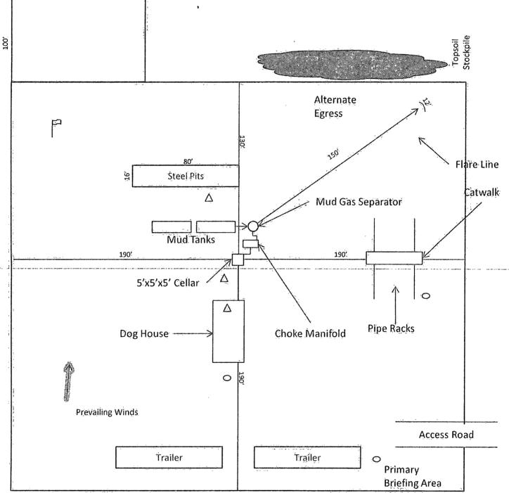
N Exhibit "D" p Wind Direction Indicators **Rig Diagram** (wind sock or streamers) **Double X 25 Federal 9**  H2S Monitors **Cimarex Energy Co.** Δ (alarms at bell nipple and shale shaker) 25-24S-32E SHL 330' FNL & 660' FWL **Briefing Areas** 0 BHL 330' FSL & 660' FWL Lea County, NM
