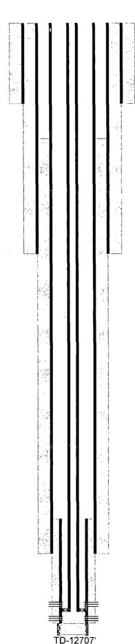
17-1/2" hole @ 1118' 13-3/8" csg @ 1118' w/ 950sx-TOC-Surf-Circ
