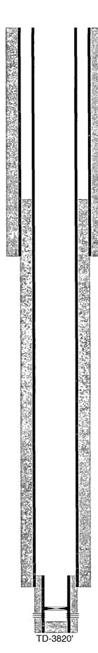
12-1/4" hole @ 1430' 8-5/8" csg @ 1430' w/ 730sx-TOC-Surf-Circ
