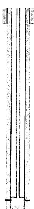
12-1/4" hole @ 380' 8-5/8" csg @ 376' w/ 200sx-TOC-Surf-Circ
