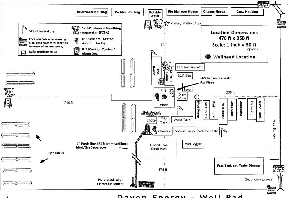
Prevailing Wind Direction S, SW Devon Energy - Well Pad Rig Location Layout Safety Equipment Location
