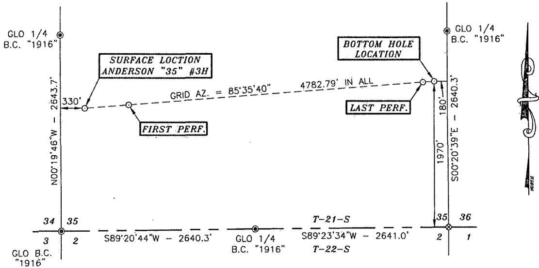
Basis of Bearings - GPS Geodetic Measurements
