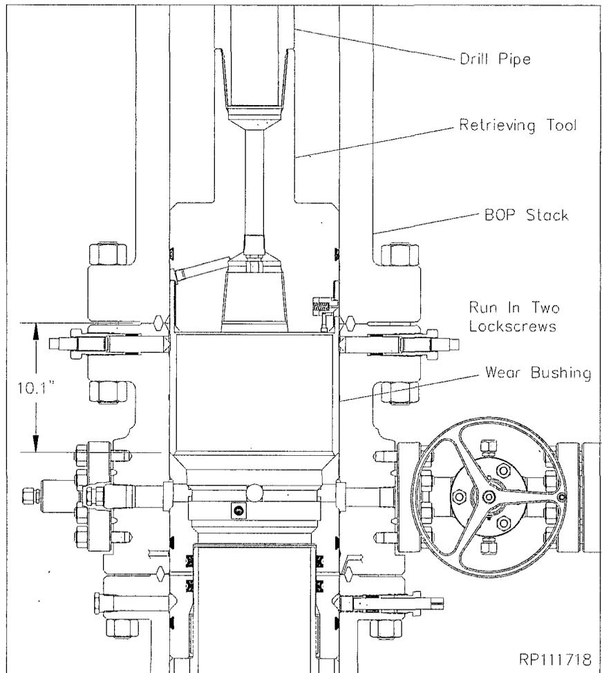
**Note:** It is highly recommended to retrieve, clean, inspect, grease, and reset the wear bushing each time the hole is tripped during the drilling of the hole section.
