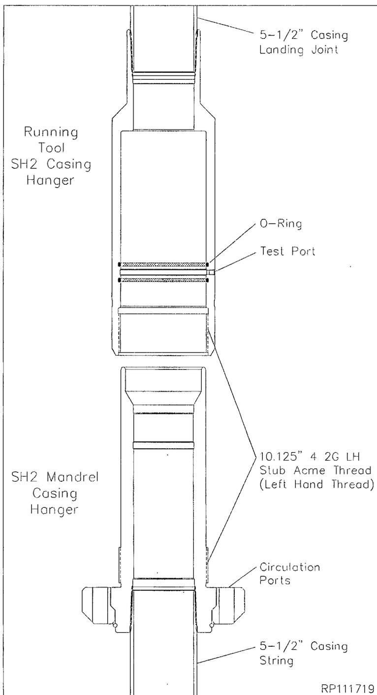
**Note:** If there is no groove present on the running tool, place a paint mark on the Running Tool as indicated.
