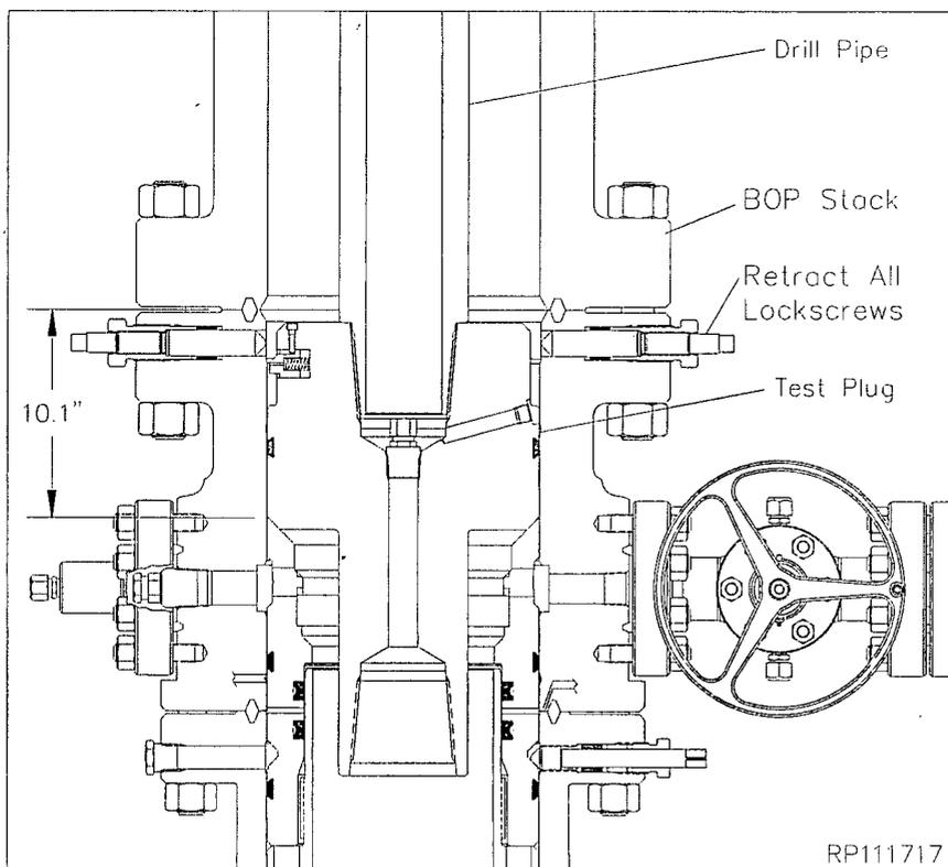
**Note:** Any leakage past the test plug seal will be monitored at the open side outlet valve.
