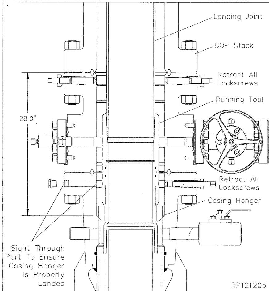
**Note:** If the casing is to be reciprocated during cementing, it is advisable to pick up the casing hanger a minimum of the length of the pup joint below the hanger plus 4 feet above the landing point. Place a mark on the landing joint level with the rig floor and then reciprocate above that point. If at any time resistance is felt, re-land the casing hanger immediately.
