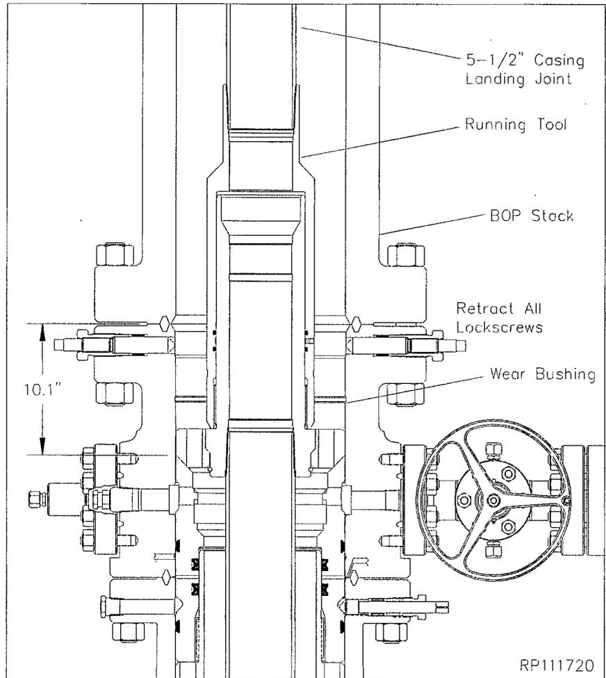
**Note:** Returns may be taken through the circulation ports and out the BOP or out the side outlets on the Casing Head.
