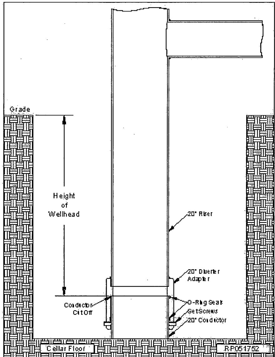
13. Prior to running the 13-3/8" casing the Diverter Riser must be removed.
