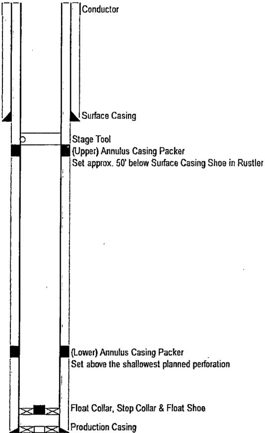
**Two-Stage Cementing (Alternative for Oil / Water / Gas & Water Flow)**
