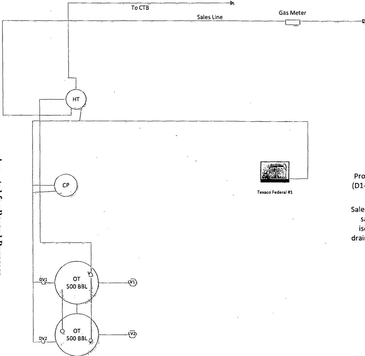
Production Phase: all drain valves (D1-D2) and sales valves (L1-L2) are sealed closed.
