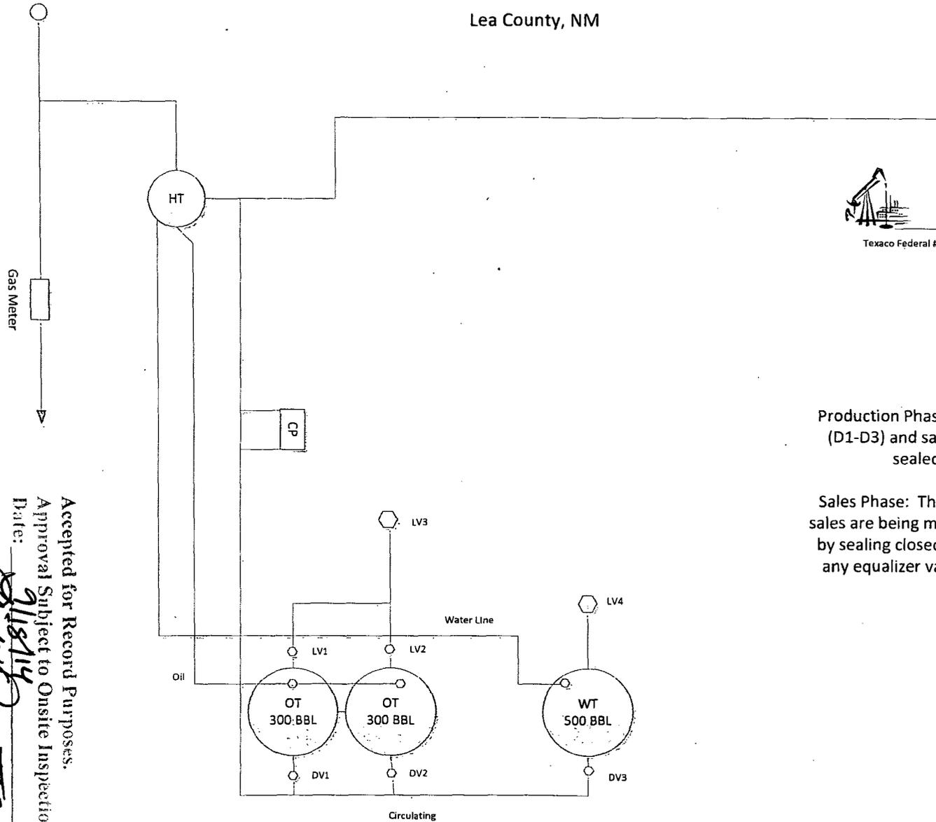
Production Phase: All drain valves (D1-D3) and sales valves (L1-L4) sealed closed.
