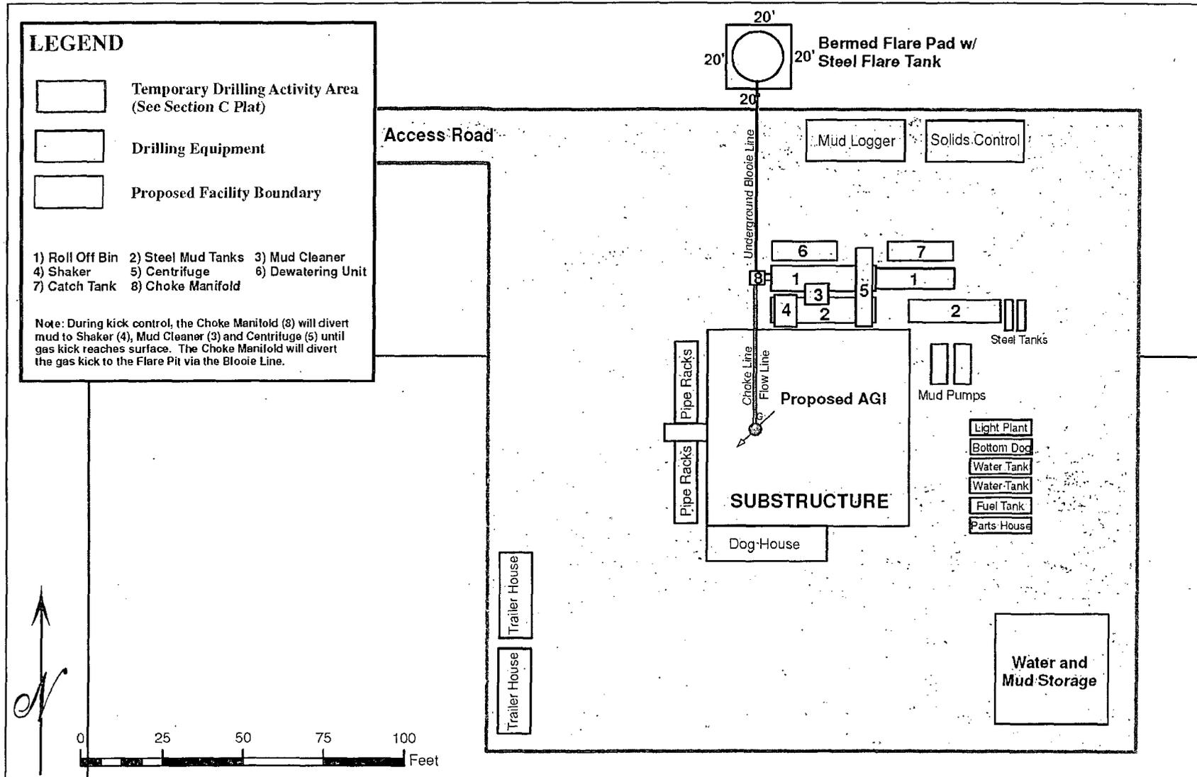
Rig Layout and Schematic with Closed Loop System Design
