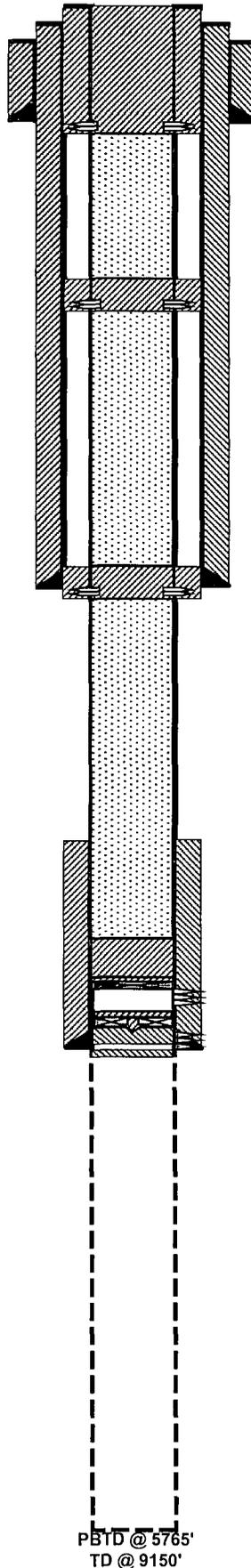
4. PUH & perf @ 349' & sqz 95 sx Class "C" cmt from 349' to surf. Attempt to CIRC 5 1/2" to surf. (Surf Shoe & Water Board)
