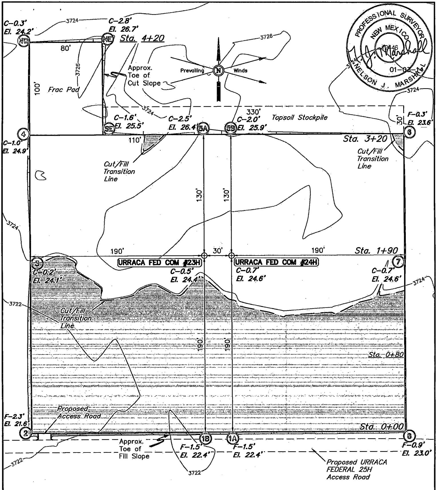
ELEV. UNGRADED GROUND AT #23 LOC. STAKE = 3724.4' FINISHED GRADE ELEV. AT #23 LOC. STAKE = 3723.9'
