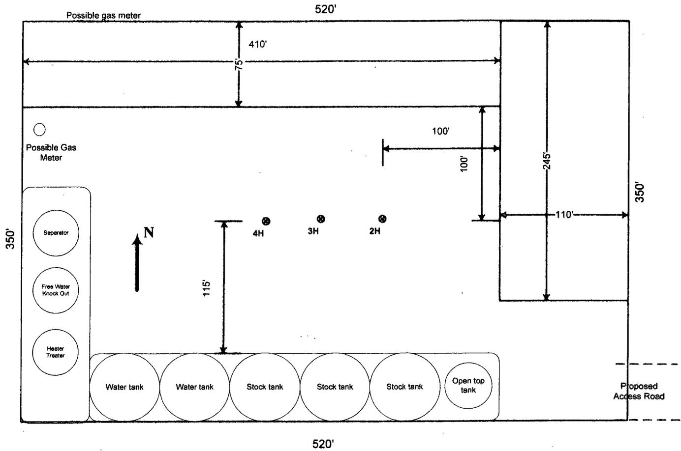
Note: A distance of 100' is required between fired vessels and any combustibles for safety purposes.
